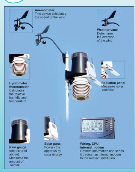
Fig. 17. Meteorological station with instruments.
